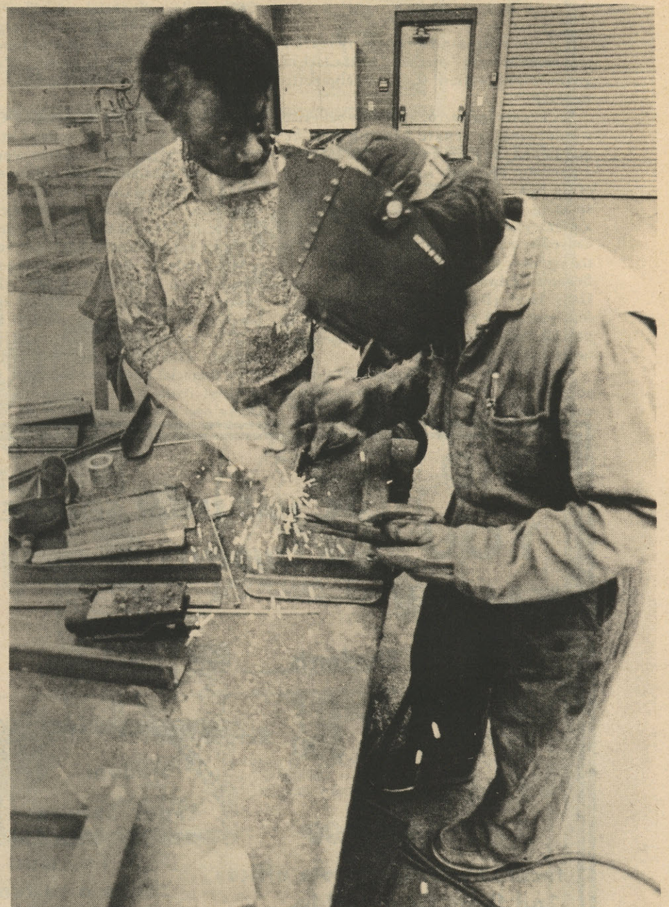
Welding majors Roy Stokes and Melvin Howard complete work on a motor mount. Stokes had to wait one entire year before getting into the program.
