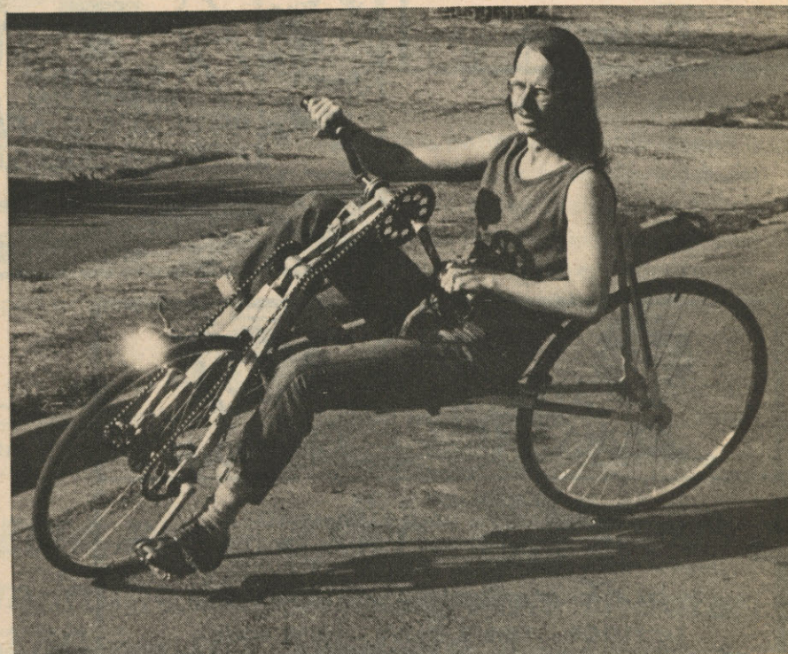
Thomas demonstrates riding his invention, which has independent hand and foot pedals, five gears, and back-pedal foot brakes. Thomas likes to use foot clips to prevent loss of energy. (Photo by Barney Kilkenry)
