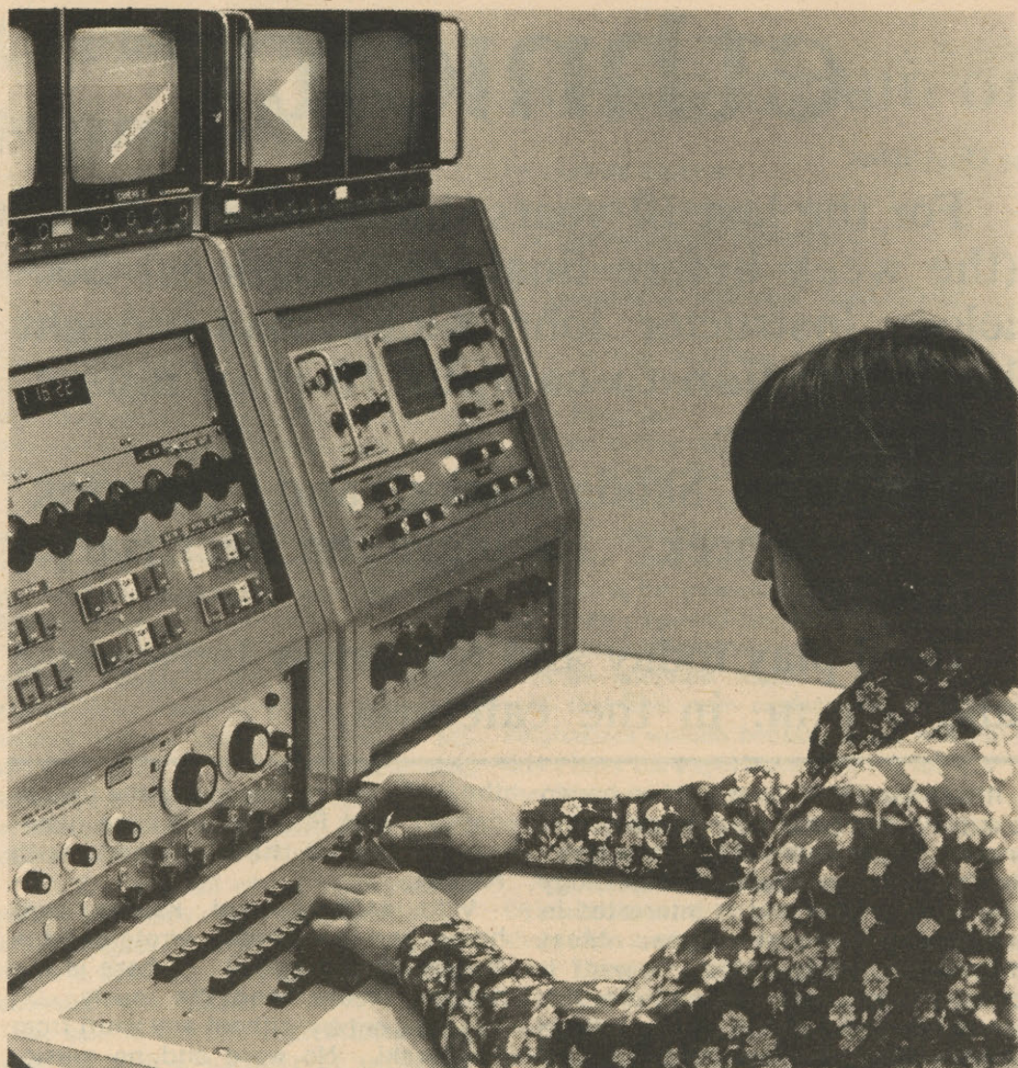
First year student Jerry Degier operates the master control switcher, which monitors picture quality.
